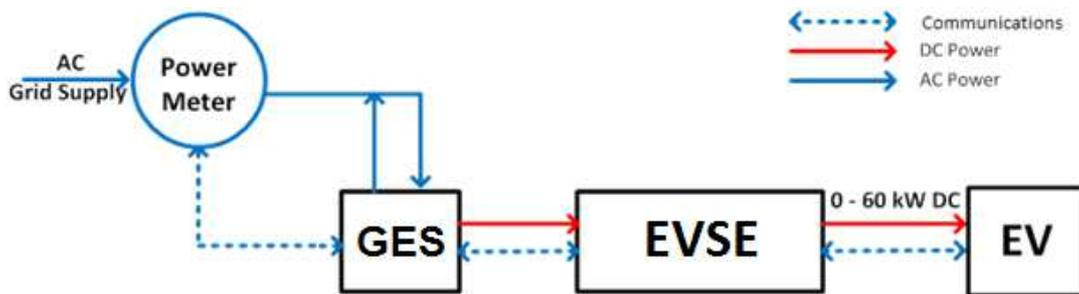
**Figure 1 - GES assisted recharging of an EVSE**
