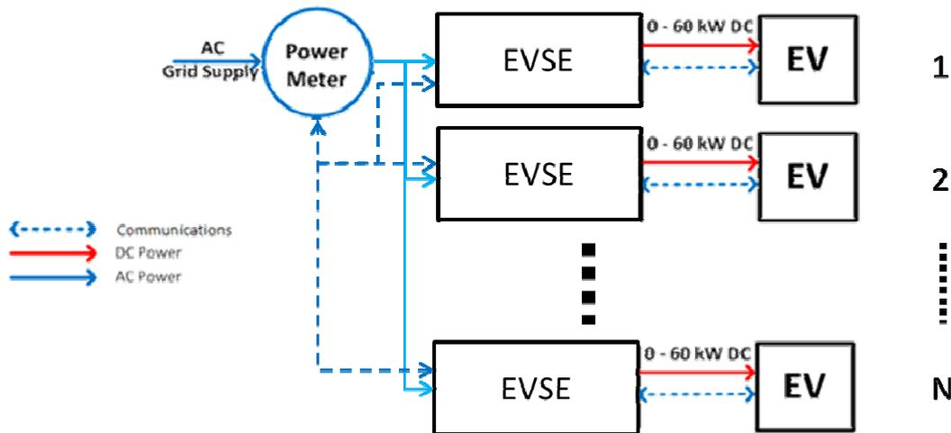
**Figure 3 – Aggregation of multiple EVSE units supplied via a single grid connection**
