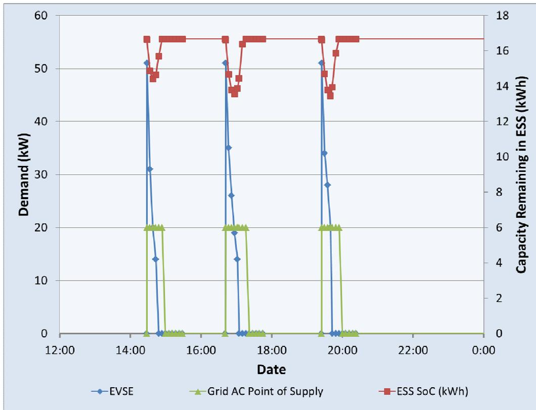
**Figure 2 – Charging and discharging a GES to support DCFC demand over a 12-hour period**
