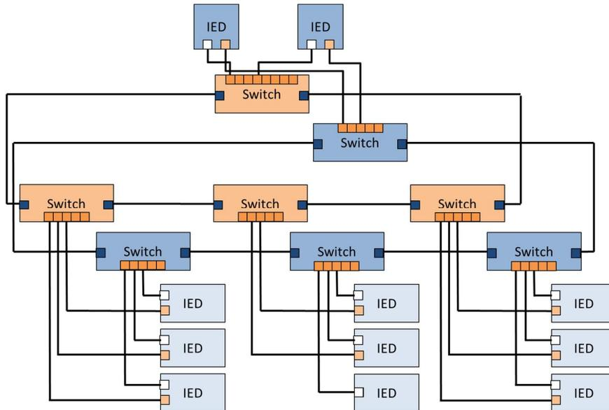
*Figure 5 – Parallel Redundancy Protocol (PRP) Configuration*
