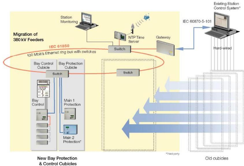
**Figure 7 – Overview of the new staged IEC 61850 substation automation system configuration [5]**
