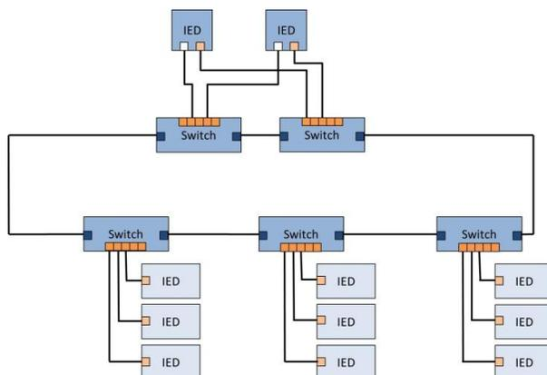
*Figure 4 – Fault Tolerant Ring Configuration*
