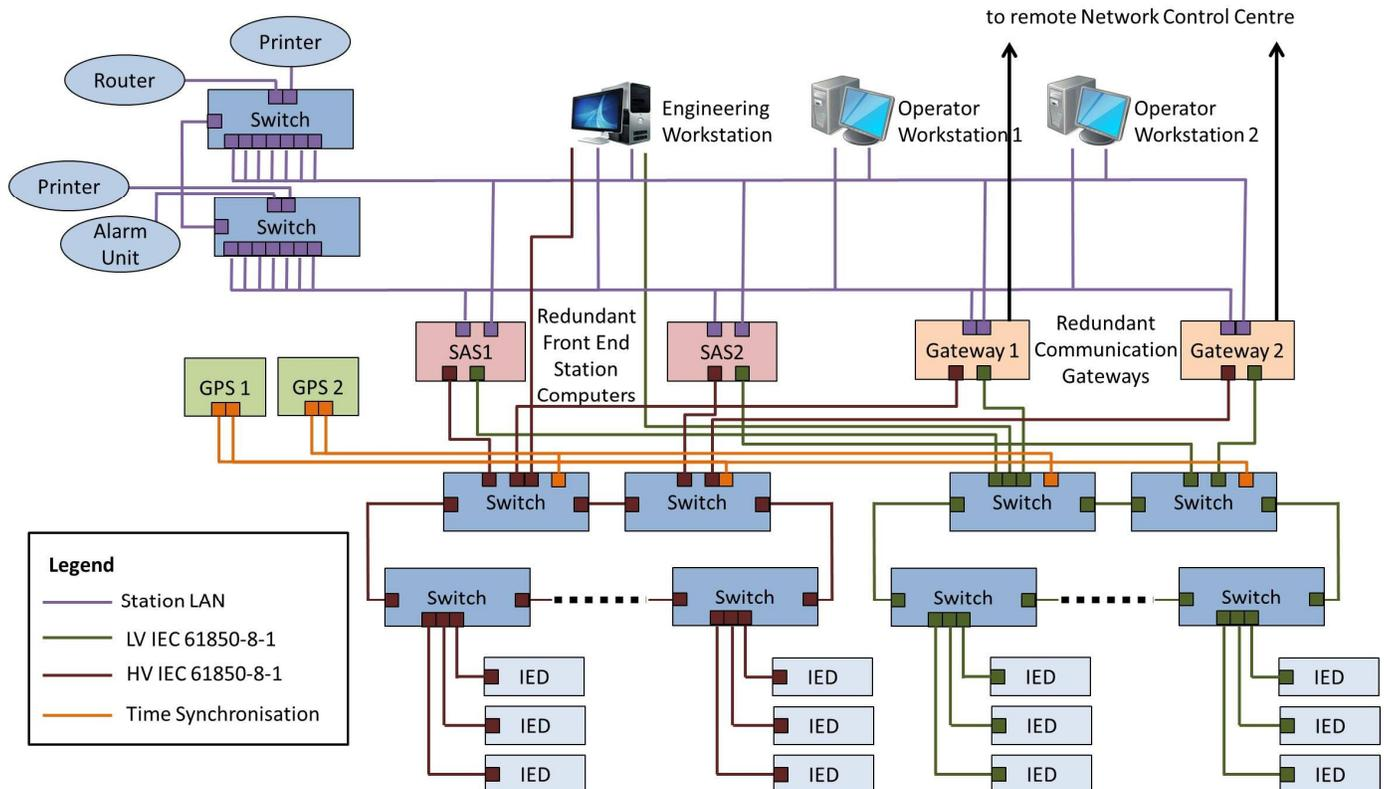
**Figure 3 – Example of an IEC 61850-8-1 Substation Automation System**
