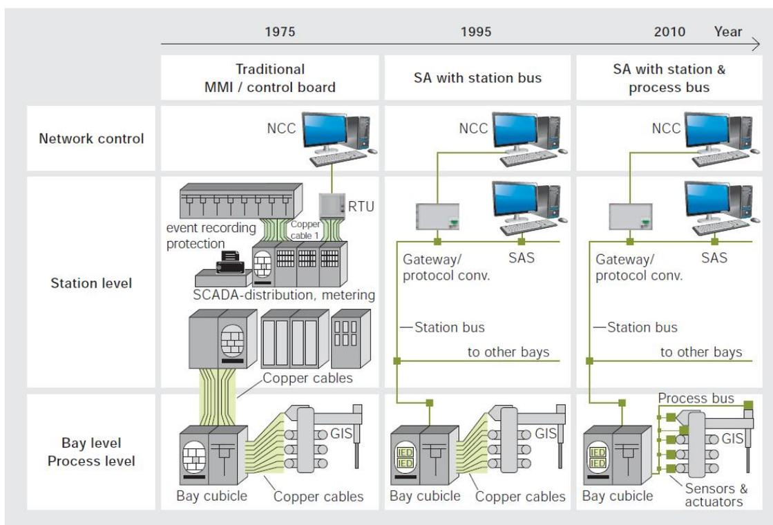
Figure 1: Development of Substation Automation Systems [1]
