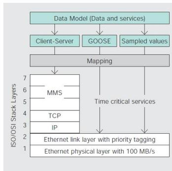
**Figure 1 – IEC 61850 Mapping to the ISO/OSI Stack [1]**
