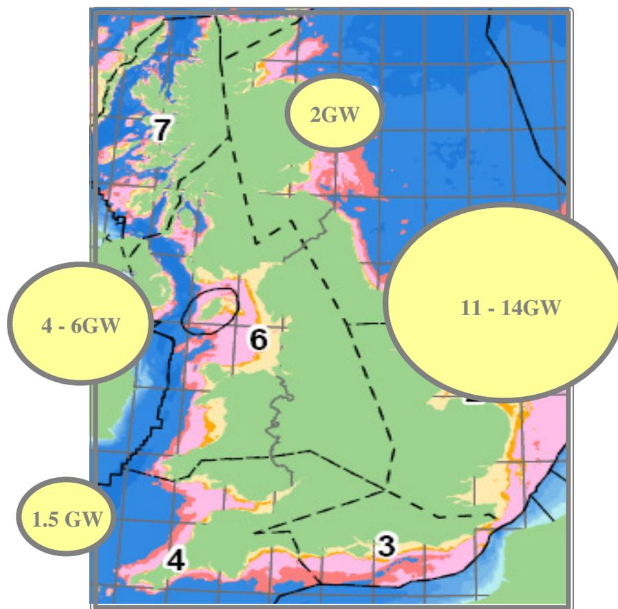
Figure 3 - Location of Potential Off-Shore Wind Farm Capacity<sup>7</sup>
