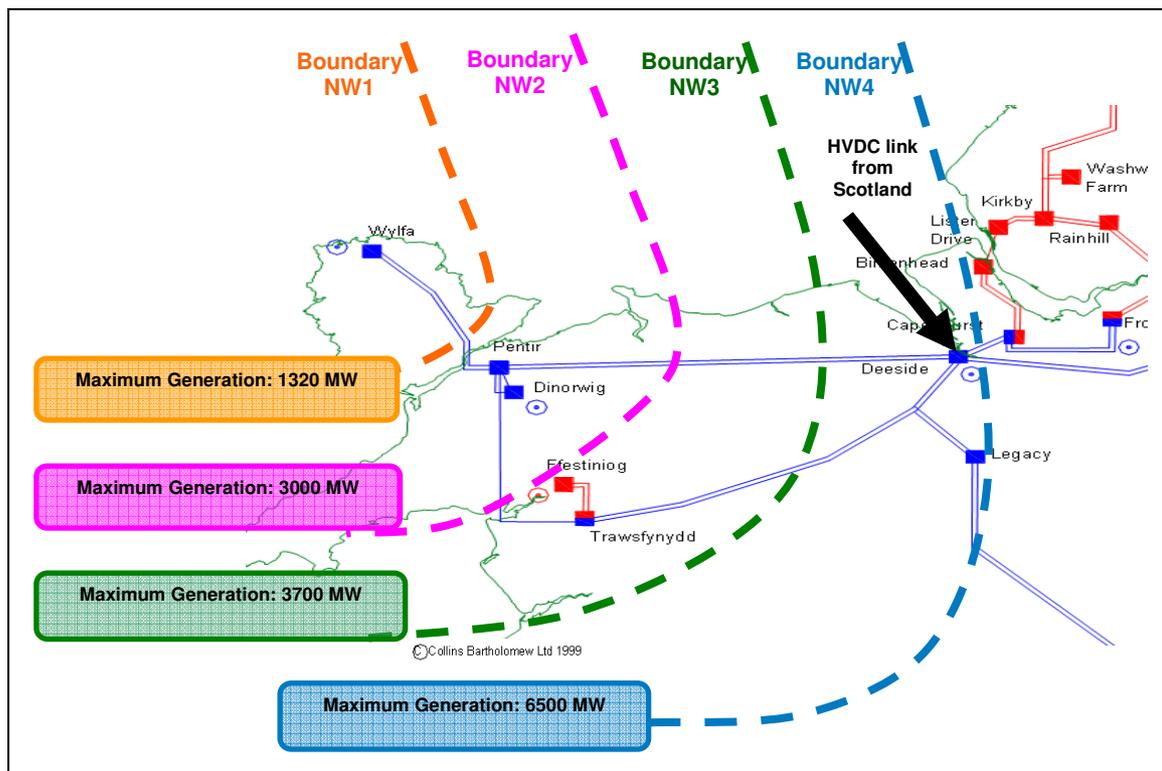
Figure 4 - North Wales Boundaries and Current Capacity Limits<sup>8</sup>
